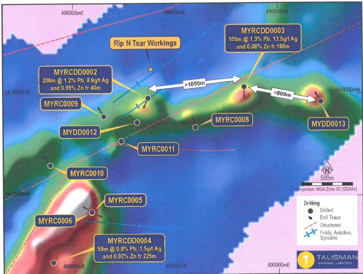
Figure 3 – Rip n Tear RC drilling over MLEM Geophysical survey image.
