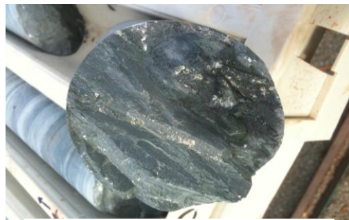
Springfield Diamond Drill Core showing Disseminated Chalcopyrite
