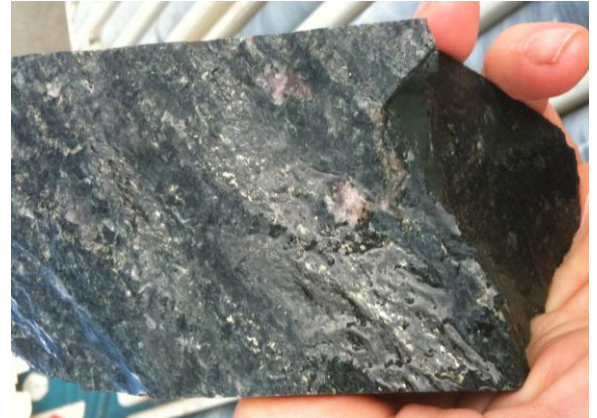
Springfield Diamond Drill Core showing Disseminated Chalcopyrite
