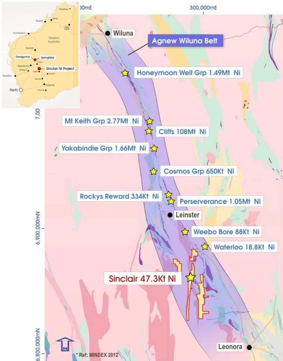
Figure 1: The Sinclair Nickel Project showing regional geology nickel production centres and reported contained nickel* of the Agnew-Wiluna Belt (*MINDEX 2012)
