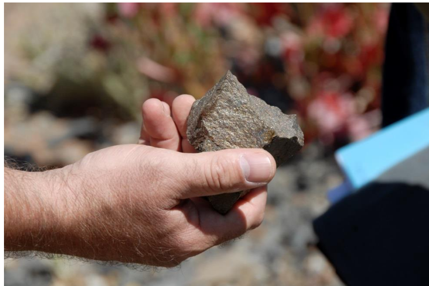
Nickel bearing massive sulphide from the Sinclair Nickel Project
