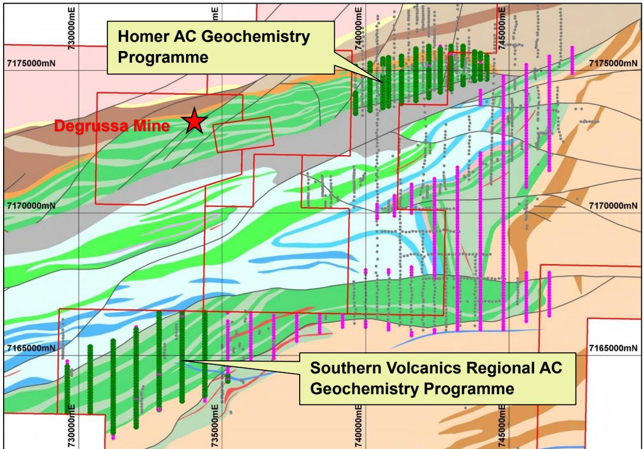
Figure 5: Springfield Project interpreted geology showing regional Aircore drill holes; completed holes in green and holes to be drilled in March 2015 Quarter in magenta.
