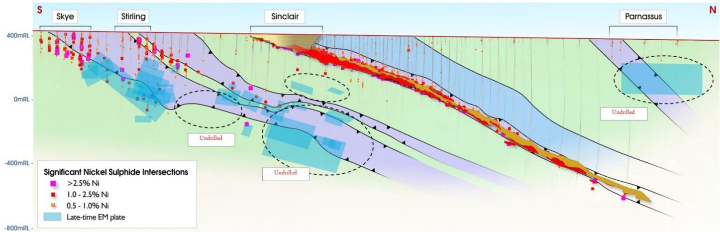
**Figure 1:** Longitudinal projection showing Stirling, Skye ultra-mafic channels, nickel sulphide intercepts, late-time EM plates in close proximity to the existing Sinclair Mine infrastructure and areas not tested by drilling.
