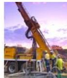
Due to the complexity of the Sinclair ore body, definition drilling needs to be closely-spaced in order to better define higher-grade shoots associated with tight folding and remobilised massive sulphide.
