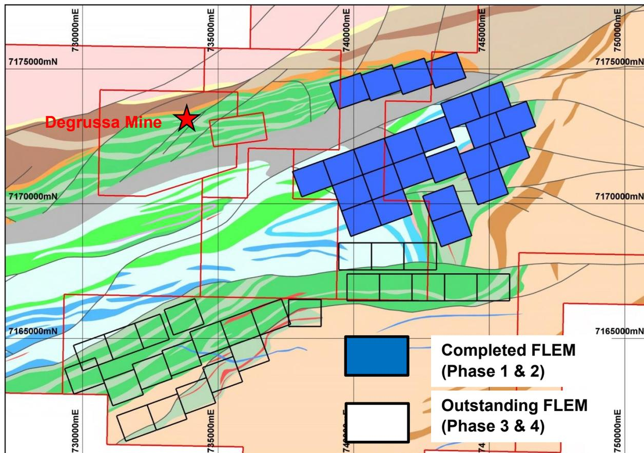
Figure 6: Springfield Project interpreted geology with Fixed Loop Electromagnetic (FLEM) survey locations; completed surveys in blue.
