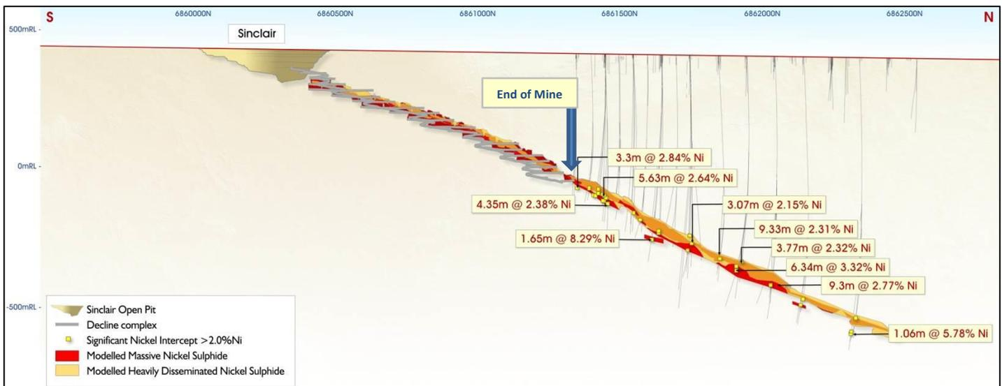
Figure 3: Sinclair Nickel deposit longitudinal projection with mine development showing mineralised Ni drill intercepts greater than 2% Ni beyond the limit of existing mine development (previously reported to ASX on 20 October 2014 – Talisman to Acquire Sinclair Nickel Project)
