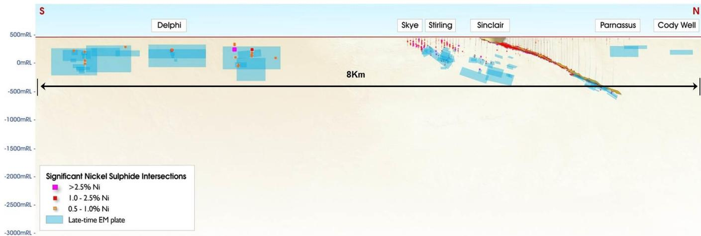
Figure 2: Sinclair Trend longitudinal projection showing 8km of strike extent, late-time EM plates and historical mineralised intercepts.
