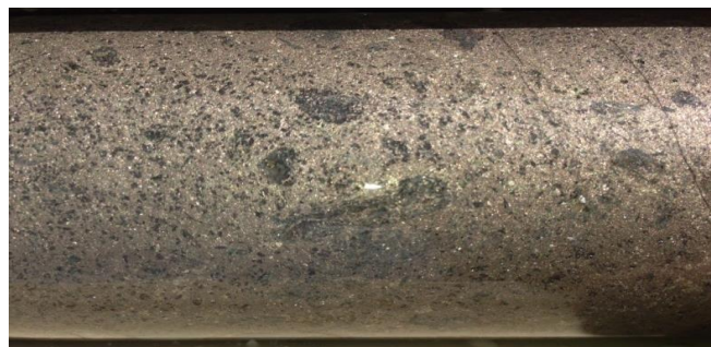
Figure 1: Massive sulphides in core from drill-hole SND001 completed in 2015 at Delphi North
