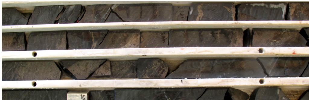
Figure 1: SND006 – Brecciated to massive sulphides (pyrrhotite, chalcopyrite & minor pentlandite) in drill core
