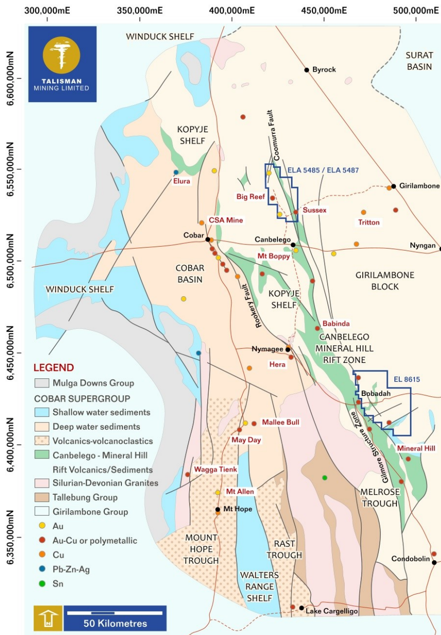
Figure 10: NSW Cobar regional geological plan, showing new TLM tenements and application locations.
