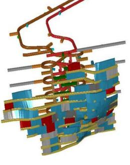
3D schematic of Monty decline and underground mine design
