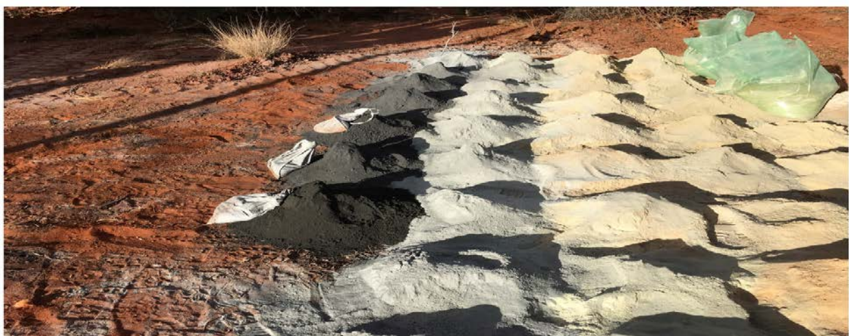
Figure 1: Skye East Prospect: SNRC048 drill cuttings showing significant intersection 51-58m 7m @3.54% Ni.
