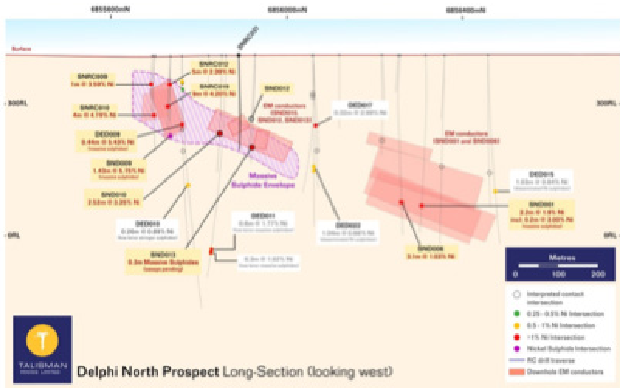
Figure 18: Delphi North projected long section showing new and existing nickel massive sulphide intersections, newly modelled (and historic) DHEM conductors, and an interpreted Massive Sulphide Envelope.
