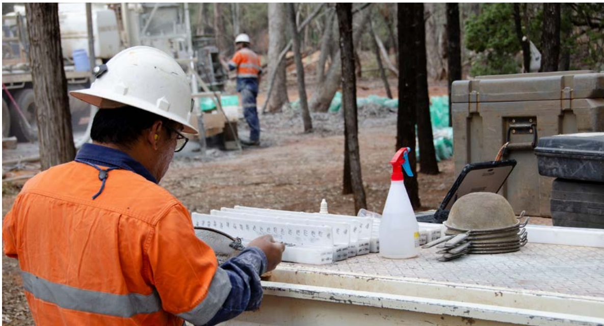
Figure 1: Logging RC drill chips at the Cumbine Prospect – Central region Lachlan Project
