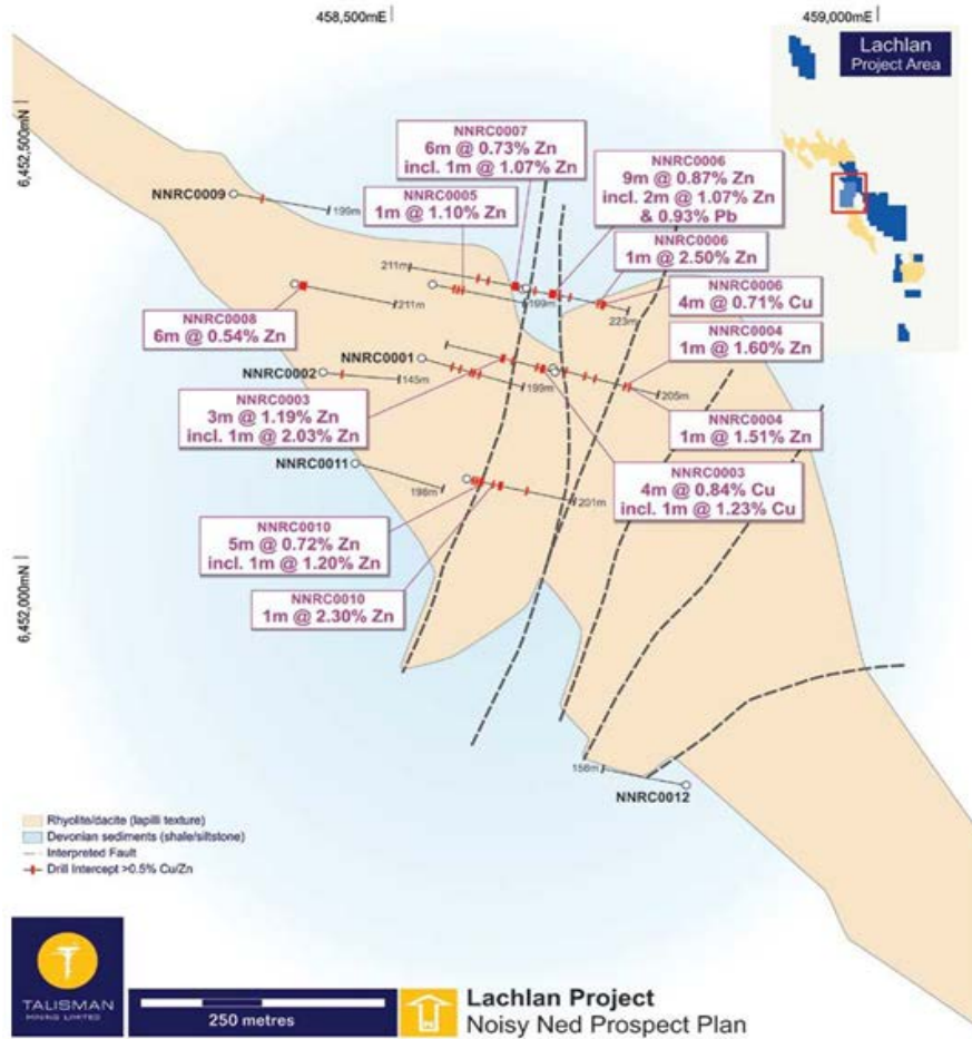
Figure 4: Noisy Ned - Drill collar locations over simplified solid geology, with RC drilling results 6
