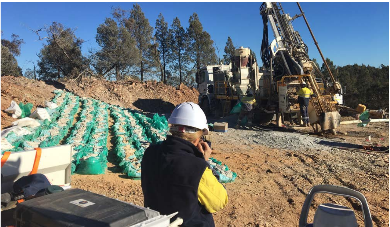
Figure 6: RC drilling and logging of chips at Blind Calf
