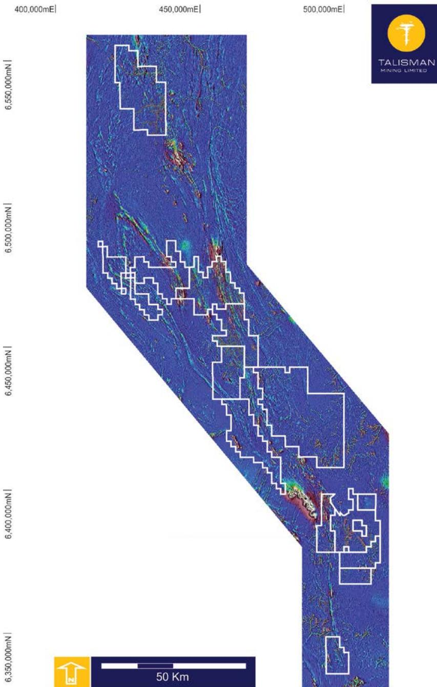
Figure 4: Lachlan Project TMI 1VD ESHADE magnetic image incorporating TLM survey data integrated with regional publicly available NSW regional data. Survey was flown on a nominal 50 line spacing and 40m height.
