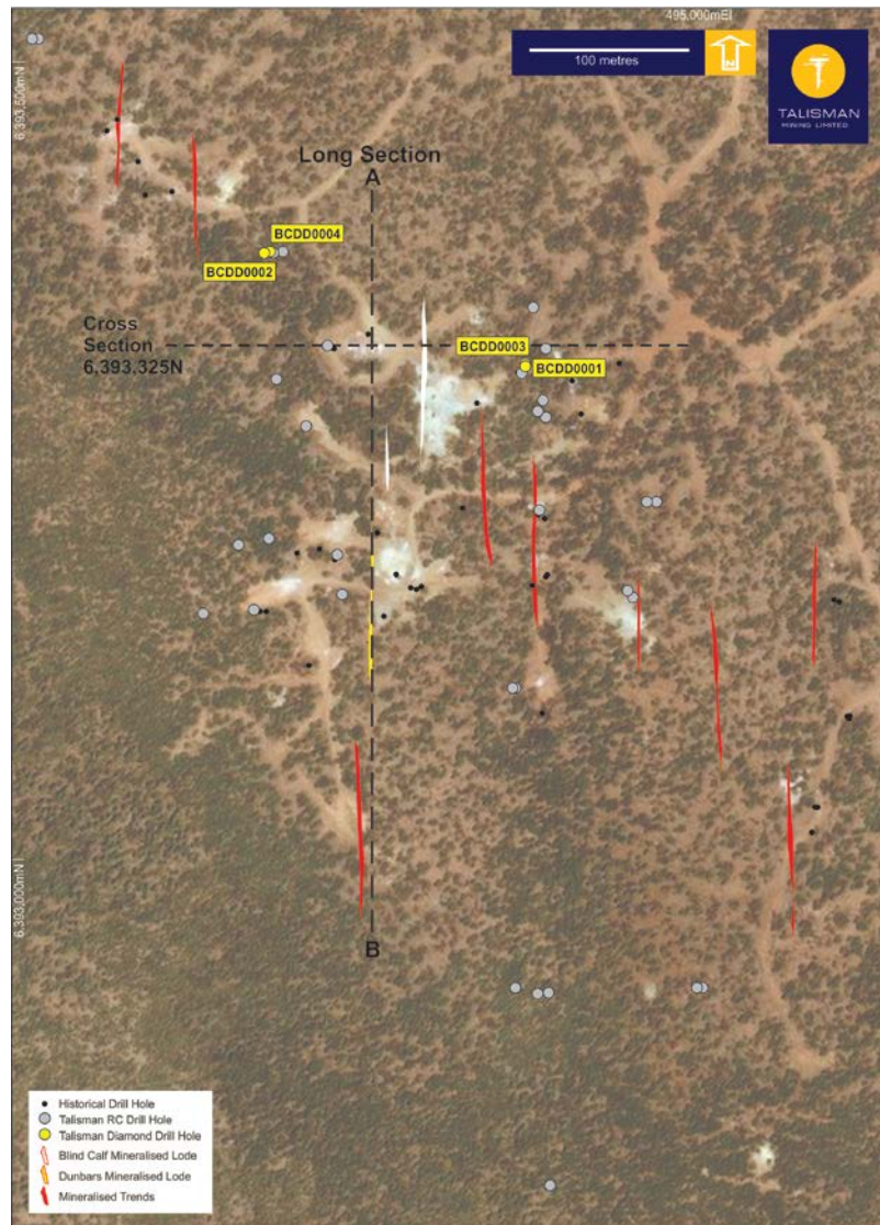
Figure 2: Blind Calf-Dunbars drill collar plan showing position of the completed diamond drill holes, including the Long Section and Cross Section positions
