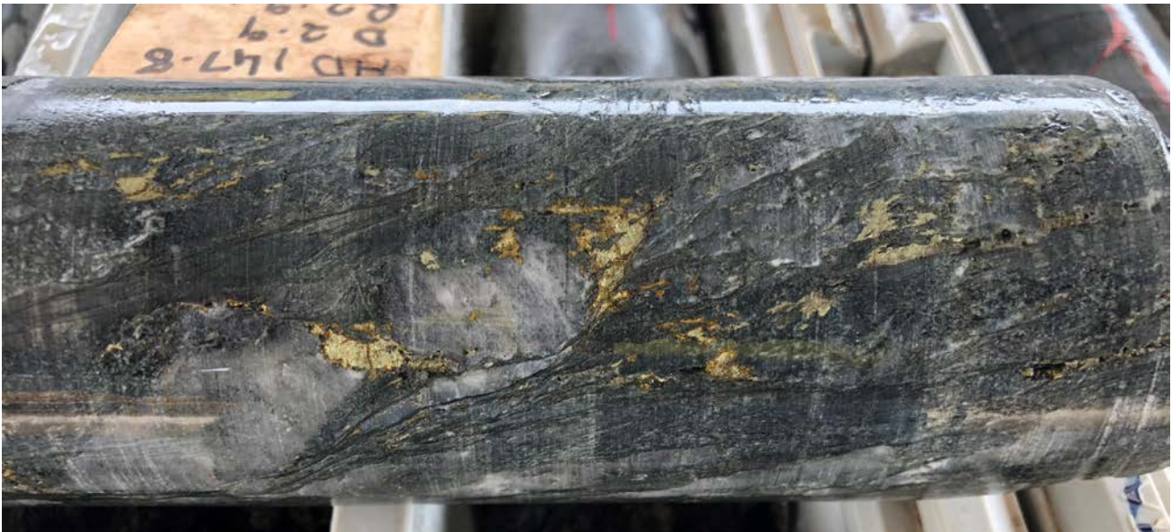
Figure 3: Blind Calf Prospect – BCDD001: Boudinage quartz sulphide vein, with sulphide mineralisation in low strain pressure shadows of quartz boudins
