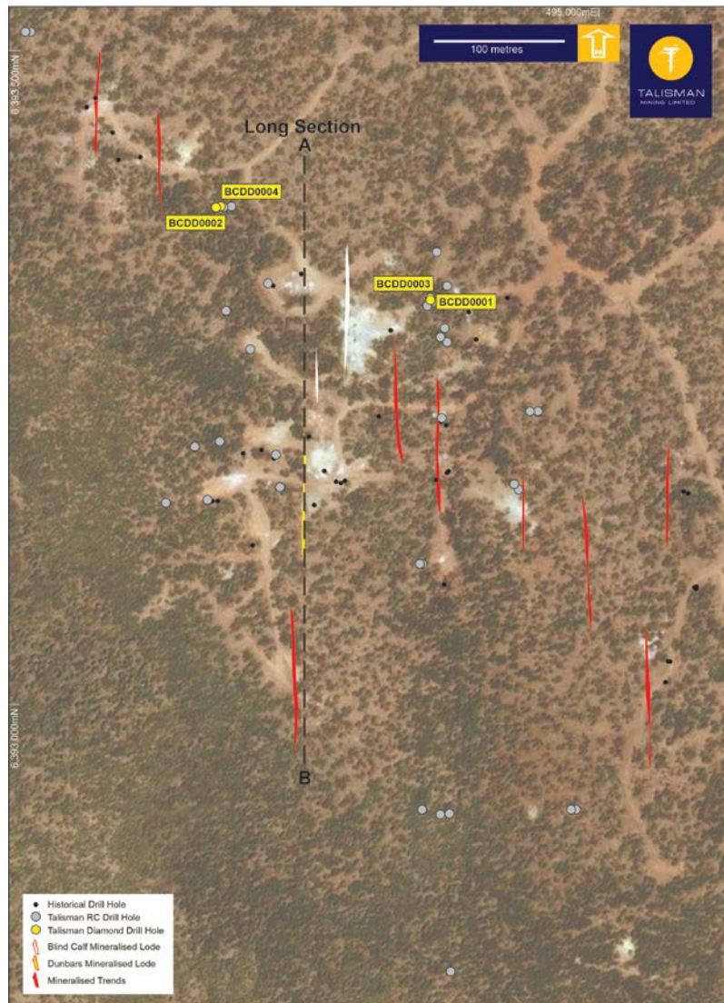
Figure 1: Blind Calf-Dunbars drill collar plan showing position of the completed diamond drill holes, including the Long Section position
