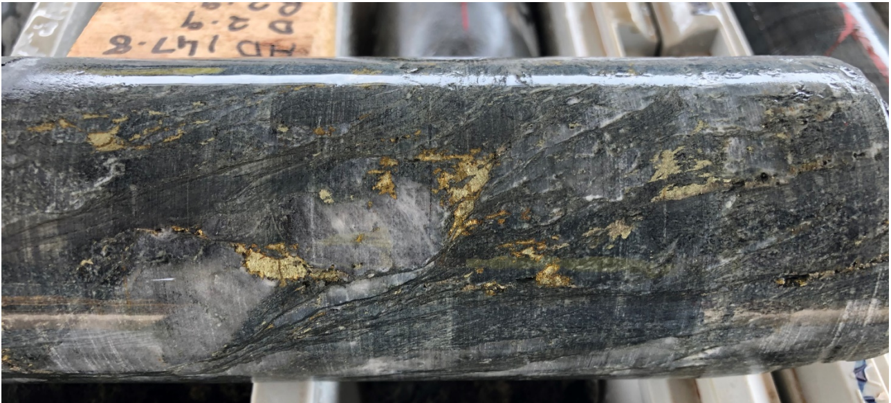
Figure 2: Blind Calf Prospect – BCDD001: Boudinage quartz sulphide vein, with sulphide mineralisation in low strain pressure shadows of quartz boudins
