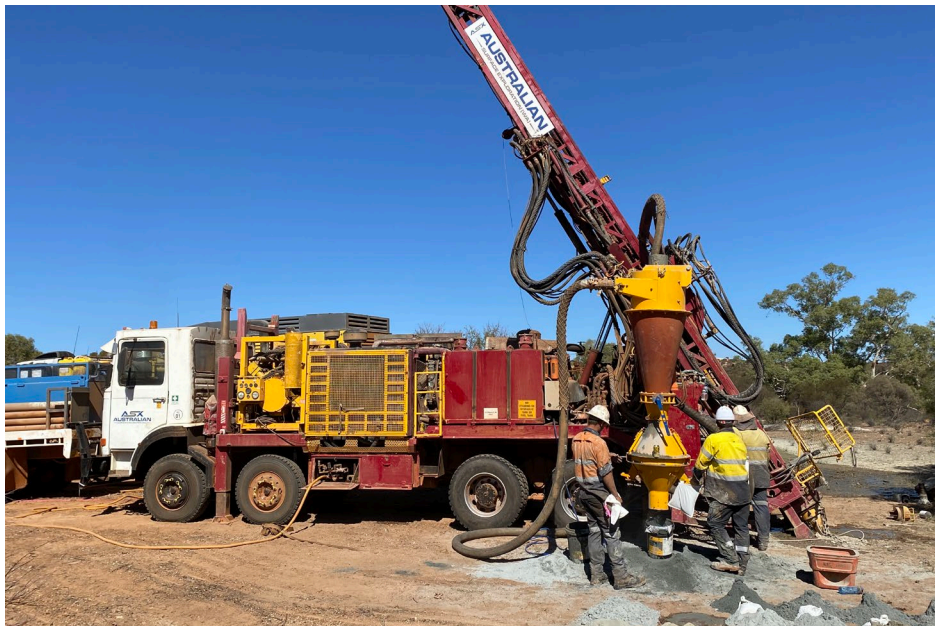
Image 1: Photo showing RC drill rig at the Ida Valley Gold Project.
