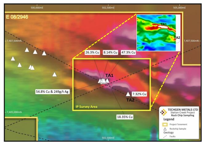
Figure 2: TA1 anomaly top right, IP survey area & interpreted faults on airborne magnetics.
