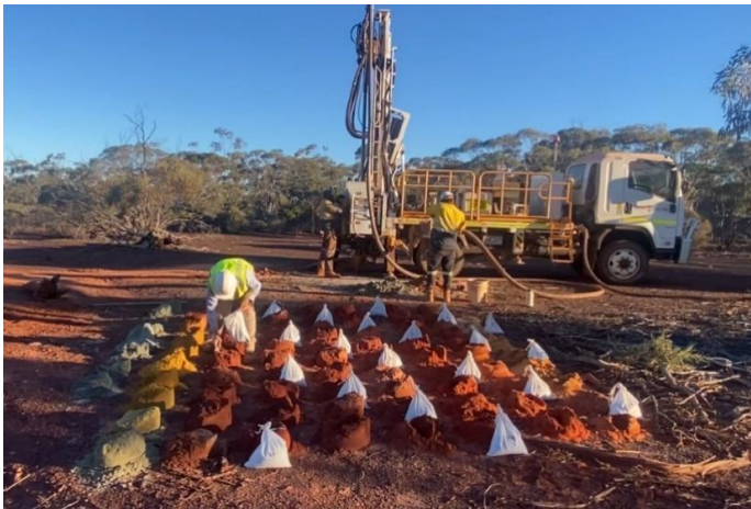
Photo 3: Star West alluvial workings and Penny's Fault aircore samples.
