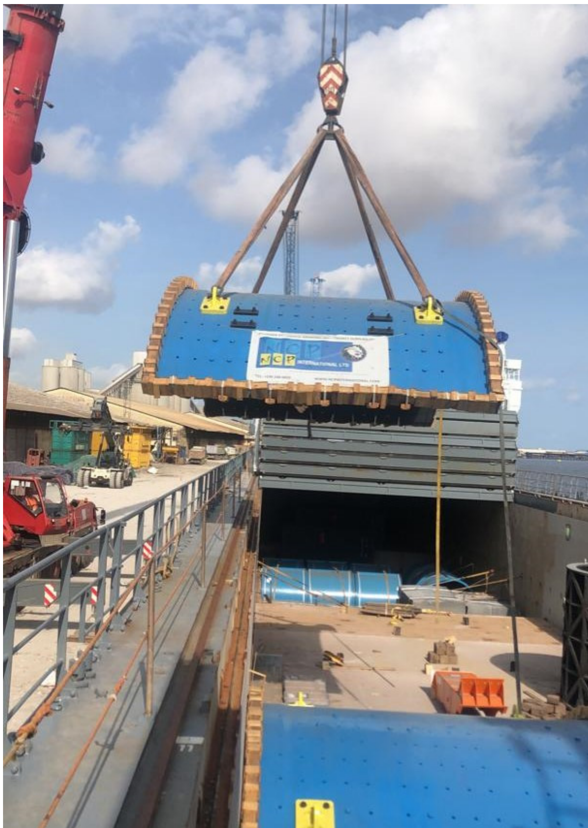
Figure 2: Abujar's SAG Mill being unloaded from the chartered vessel at Abidjan Port, Côte D'Ivoire, on 5 th June
