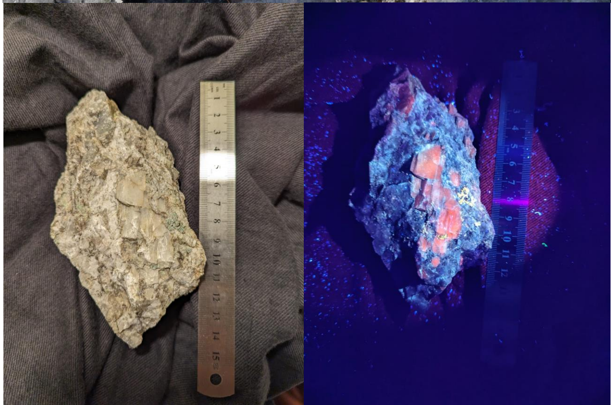
Figures 3 and 4. Field outcrop of spodumene bearing pegmatite and type samples of the spodumene bearing pegmatite found at Ross Lake in natural (left) and under UV (right). The spodumene shows as orange/red luminescence under long wave length UV light.
