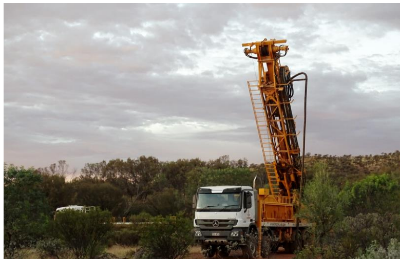
Figure 3. RC Drilling at Mount Hardy.
