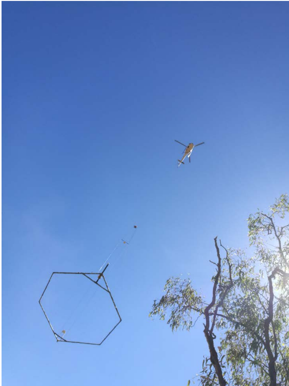
Figure 2. SkyTEM system in operation in the Northern Territory showing the helicopter and EM loop
