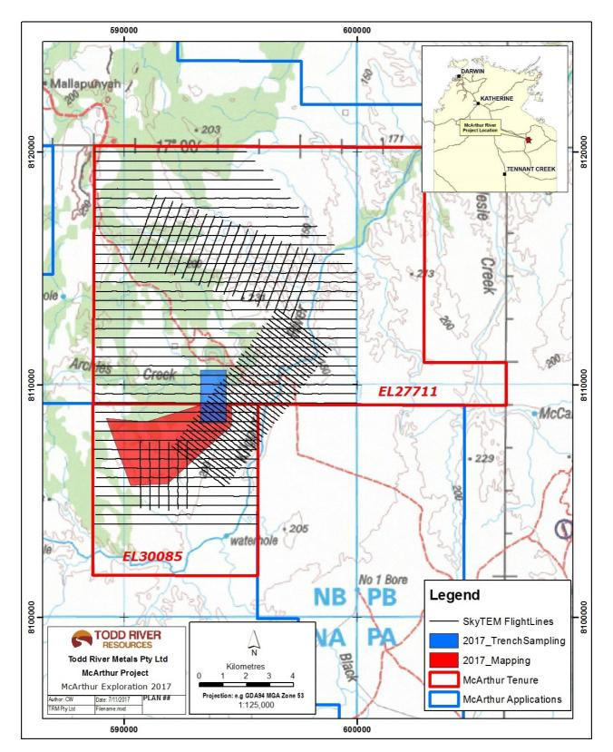
Figure 1. Location of the McArthur River Project, showing the area mapped, the rock and trench sampling area, The SkyTEM survey area, and adjoining new tenure. Figure 3 below covers the area outlined in the blue rectangle.
