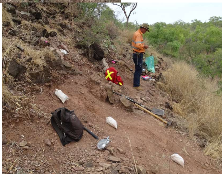
BELOW Figure 5. Channel #01 sampling, showing the Pto1/Pto2 contact (grey Pto2 dolomite LHS) and breakaway slope exposing Pto1 red/brown weathered shales.
