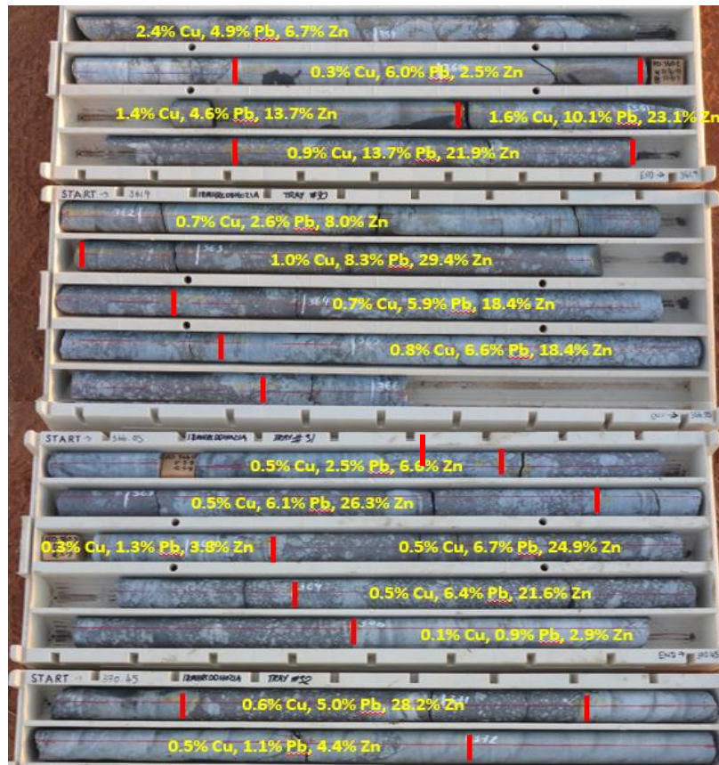
Upper stringer zone produces strong, easy to model signal
