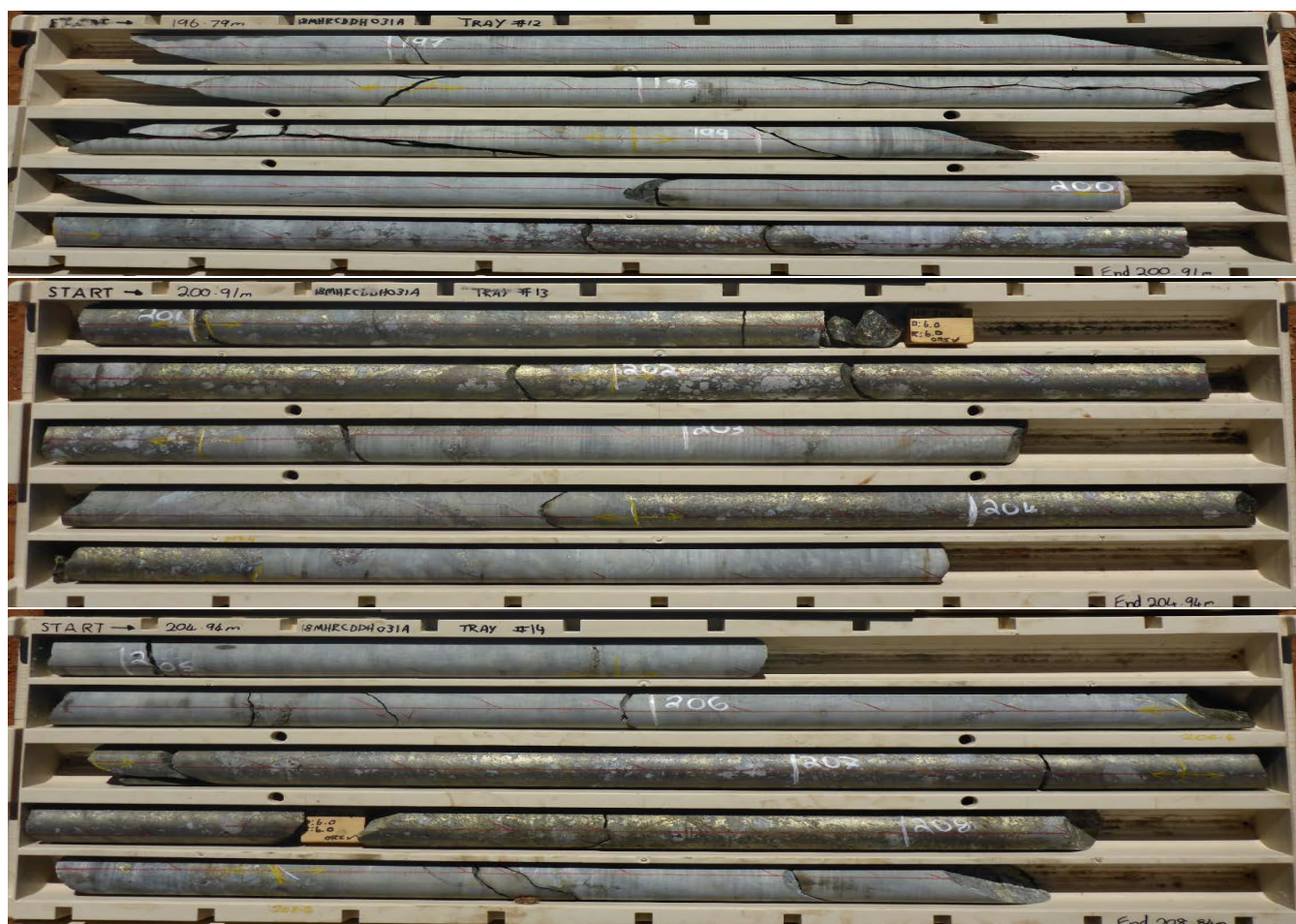
Figure 4. Drill core from MHDD0031A, showing the sulphide mineralisation from 196.8m to 209m depth. Yellow shiny core is chalcopyrite, while darker intervals are sphalerite-dominated.
