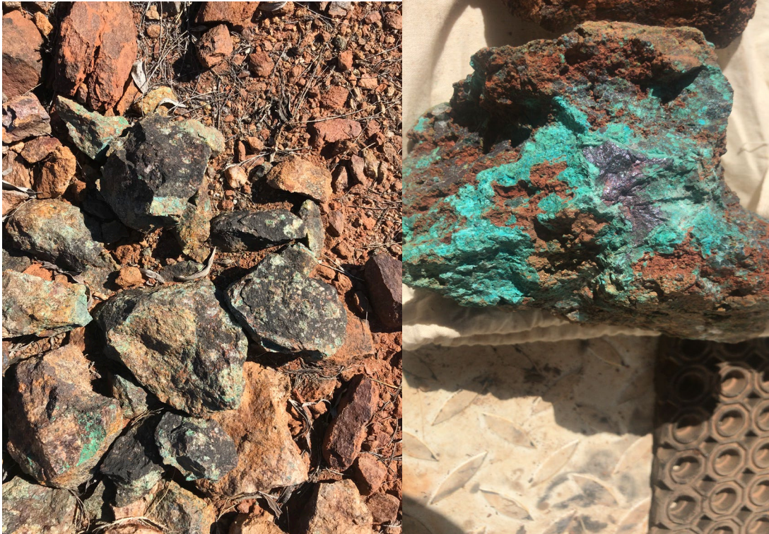
Figure 4 – photos of gossanous material and oxide copper taken from the Linda-Jane Prospect
