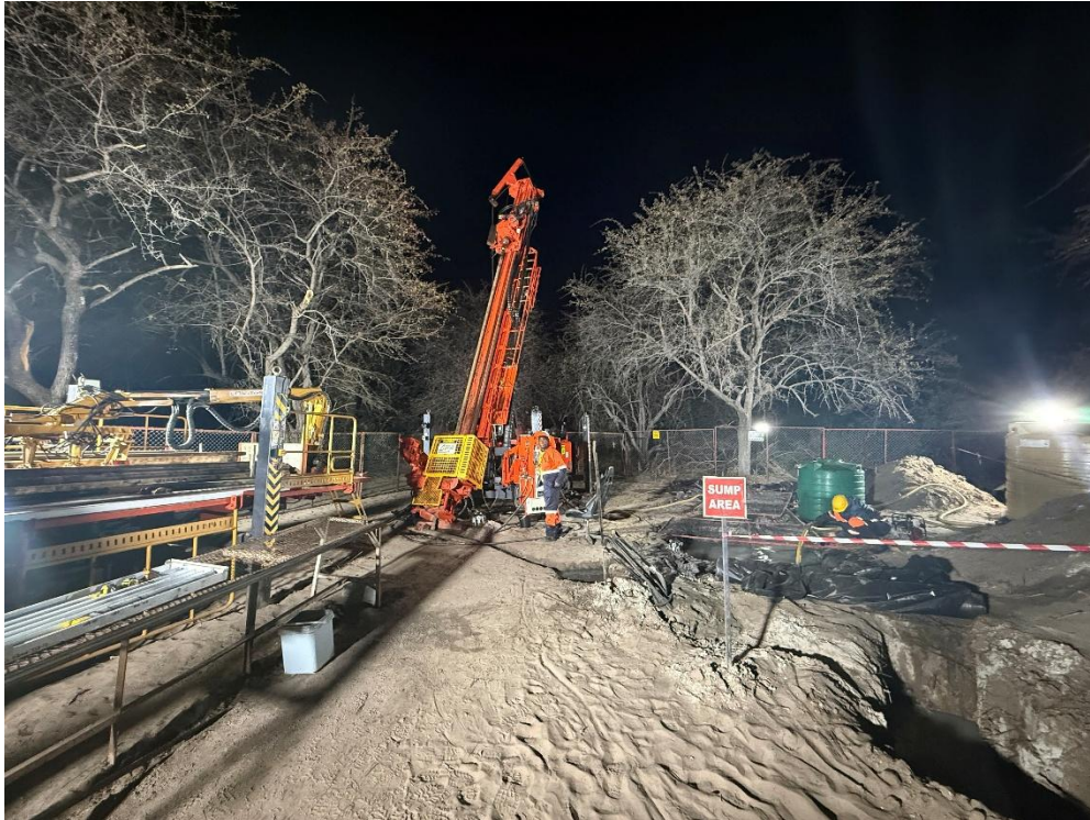
Figure 3: Diamond drilling rig at the Chanoga Prospect, KCP
