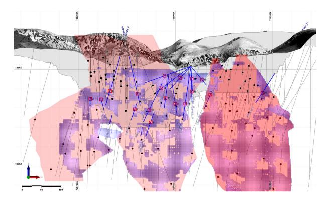
**Figure 2:** Sulphur Springs drilling Long Section with proposed Open Pit Shell, inferred (Blue) Resource Blocks and planned in-fill drill holes (blue).
