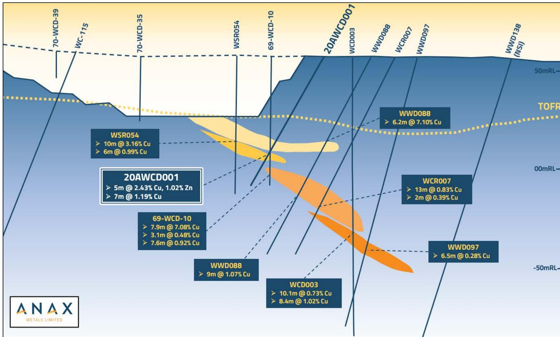
Figure 4: Oblique cross section (looking towards 305°) showing 20AWCD001, select previous drill holes and interpreted copper domains. Refer to Figure 1 for approximate cross section location. Note: A number of holes have been omitted from the section for ease of display.
