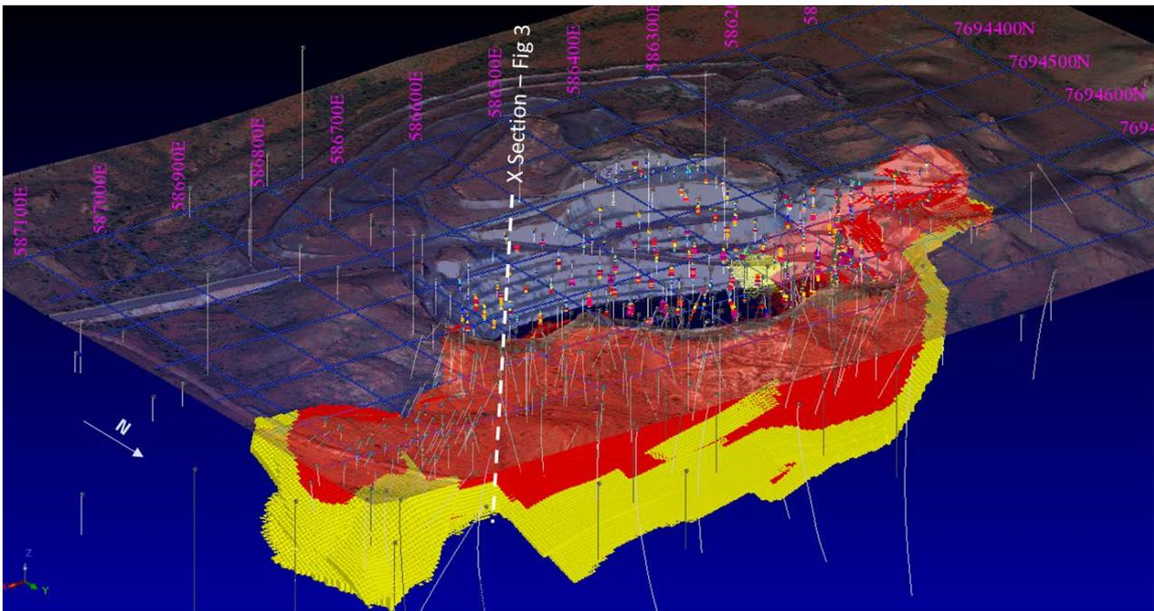
**Figure 2: Oblique view of the Whim Creek Deposit showing Indicated (red) and Inferred (yellow) resources.** View Direction is  $-25^{\circ}$  towards  $215^{\circ}$ . Figure 3 Cross Section orientation shown.
