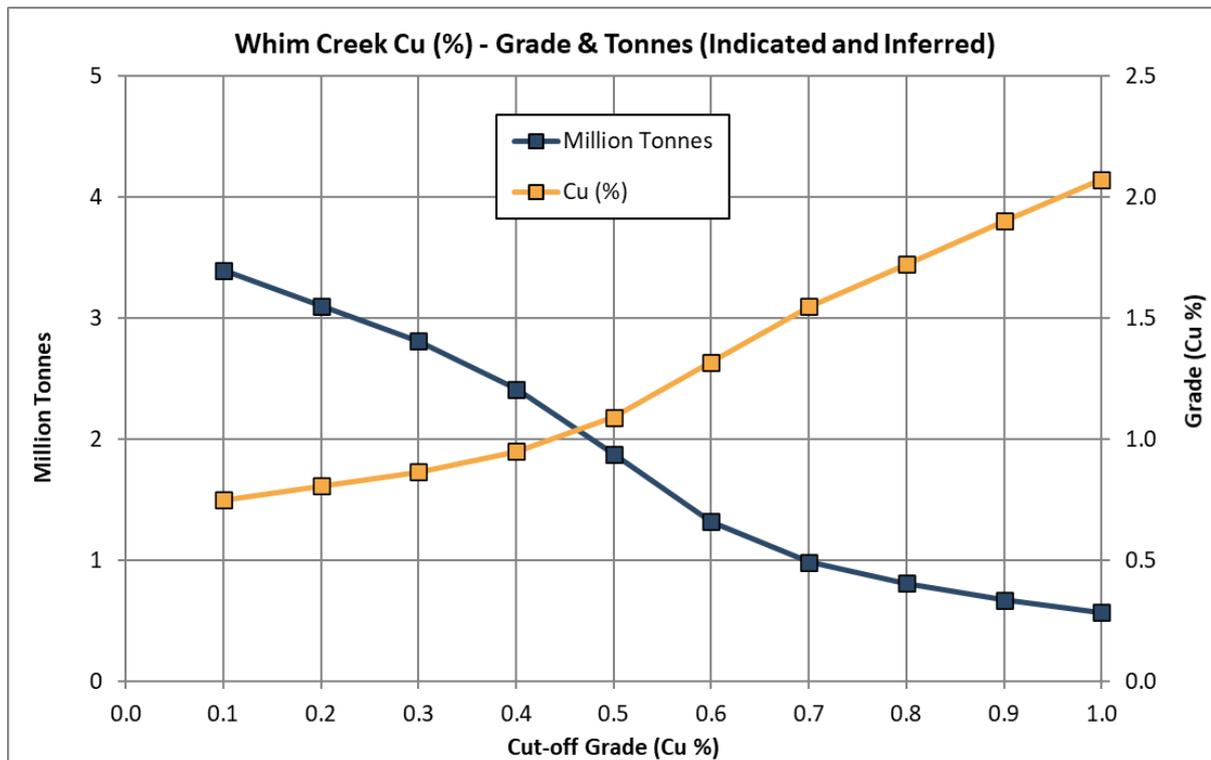
**Figure 1: Grade-Tonnage Curve based on Cu cut-offs for the Whim Creek Deposit Mineral Resource.**
