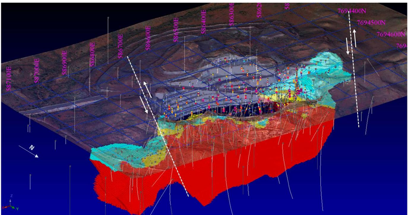
*Figure 3: Oblique view of the Whim Creek Deposit showing oxide (light blue), transitional (yellow) and fresh sulphide (red) resources. View Direction is  $-25^\circ$  towards  $215^\circ$ .*
