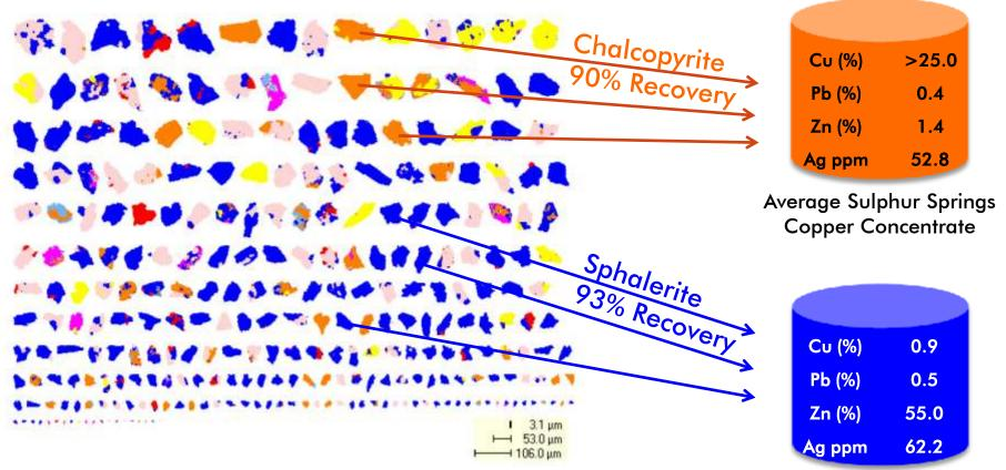
Figure 7: QEMSCAN<sup>TM</sup> mineral maps of particles analysed by SMS, for size fraction -106/+53 for sample SSP17. Total population of particles = 282. Particles sorted in order of Area.
