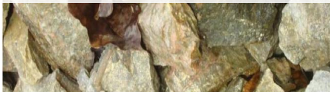
Intensely sericitised, silicified Granite and vein material Doca Prospect Shaft
