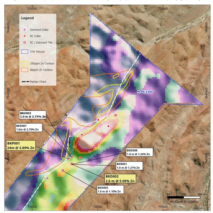
Figure 2: Breakers Prospect (Panorama Trend) with historic drilling intercepts (see asx release 9 June 2014) overlying VTEM image.
