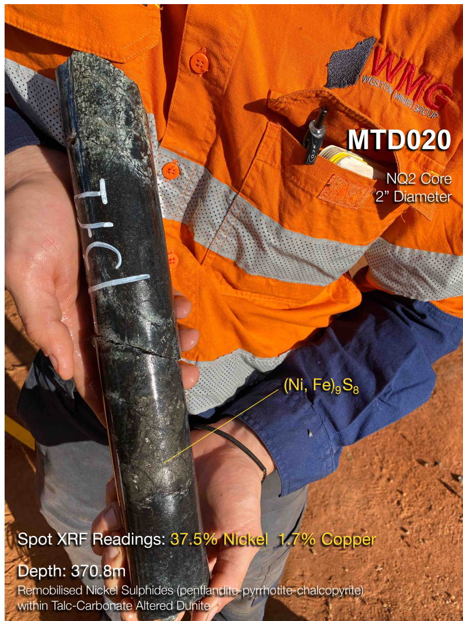
Figure 1: Photo showing examples of visible sulphides in hole MTD020
