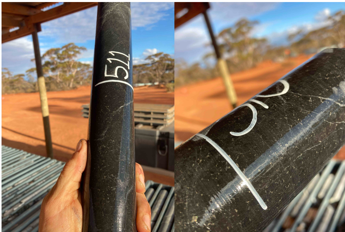
Figures 2A and 2B: Photo showing examples of visible sulphides in hole MTD020 with disseminated sulphide forming interstitial blebs between olivine grains
