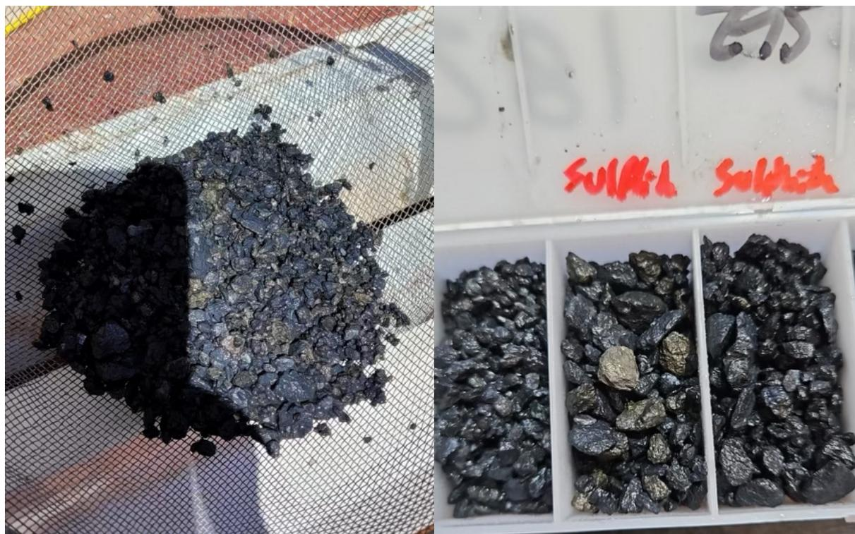
Figure 9: Photos of semi-massive sulphide chips (30-40% sulphide) MTRC018 293-294m
