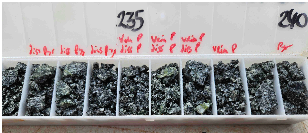
Figure 2: MTRC059 heavily disseminated and veined pyrite in granodiorite rock chips
