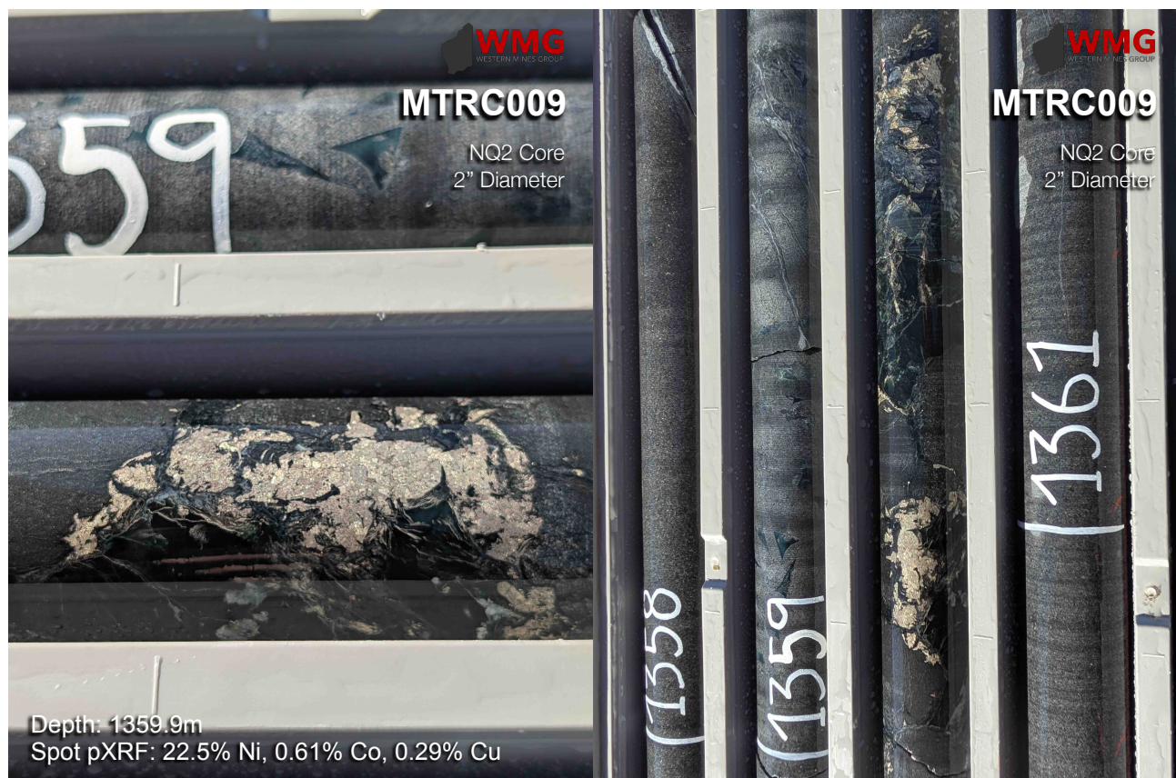
Figure 2: Photos showing examples of sulphide segregations in hole MTRC009 (EIS9)
