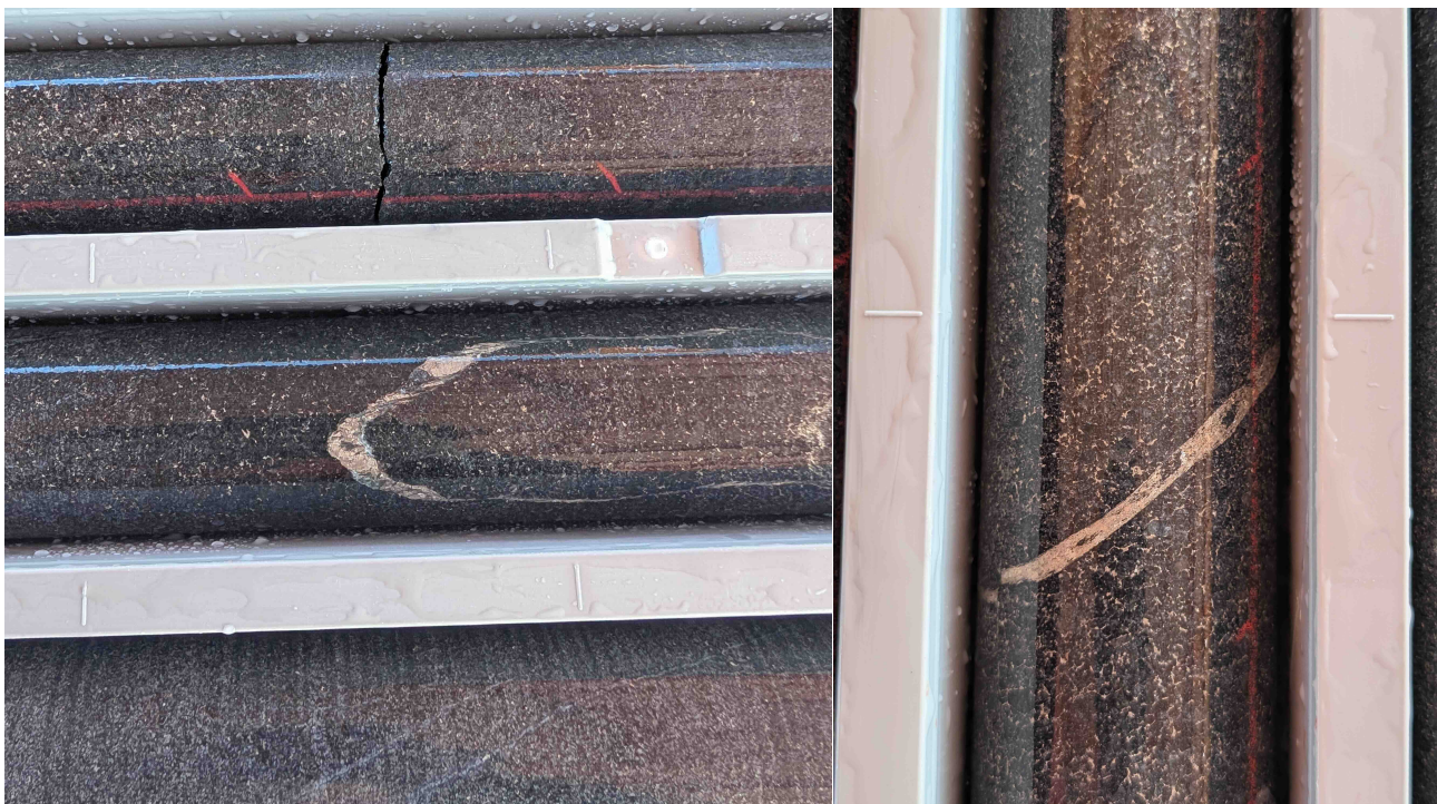
Figure 4: Photos showing examples of heavily disseminated sulphide in hole MTRC009 (EIS9) (left 1355m, right 1350m) Note: core is NQ2 being 2 inches or 50mm diameter
