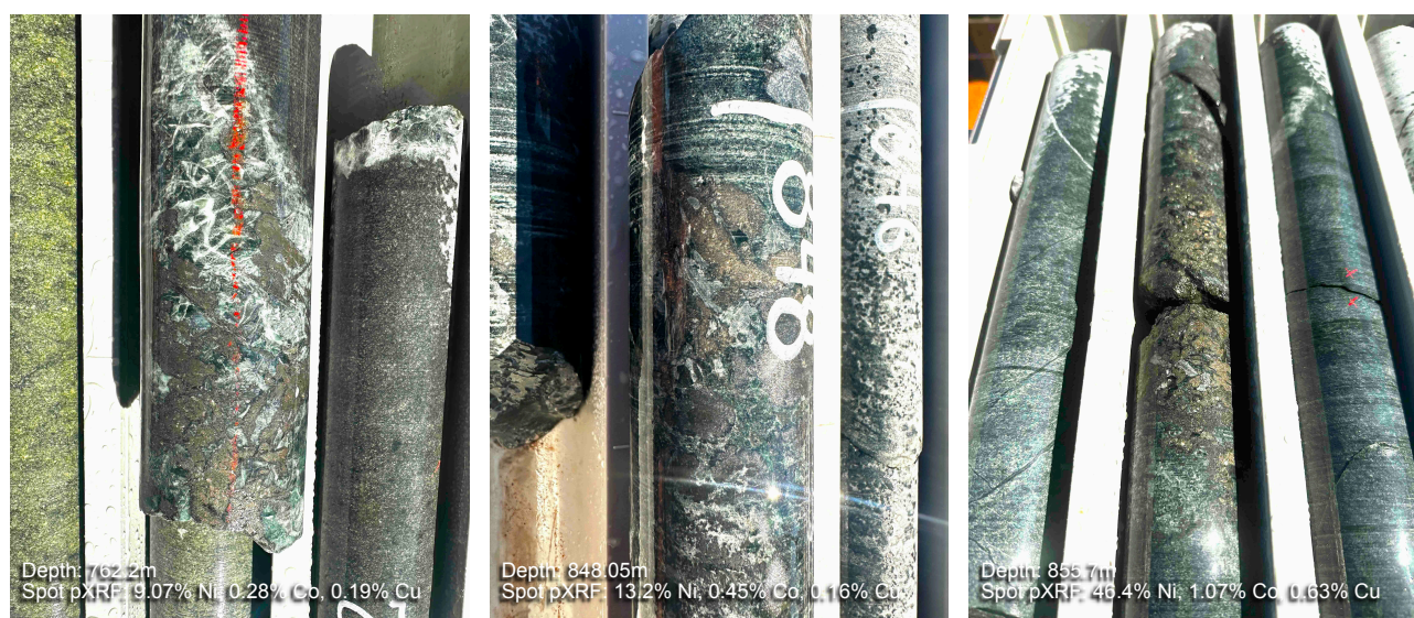
Figure 1: Photos showing examples of semi-massive sulphide segregations and globules in hole MTRC011
