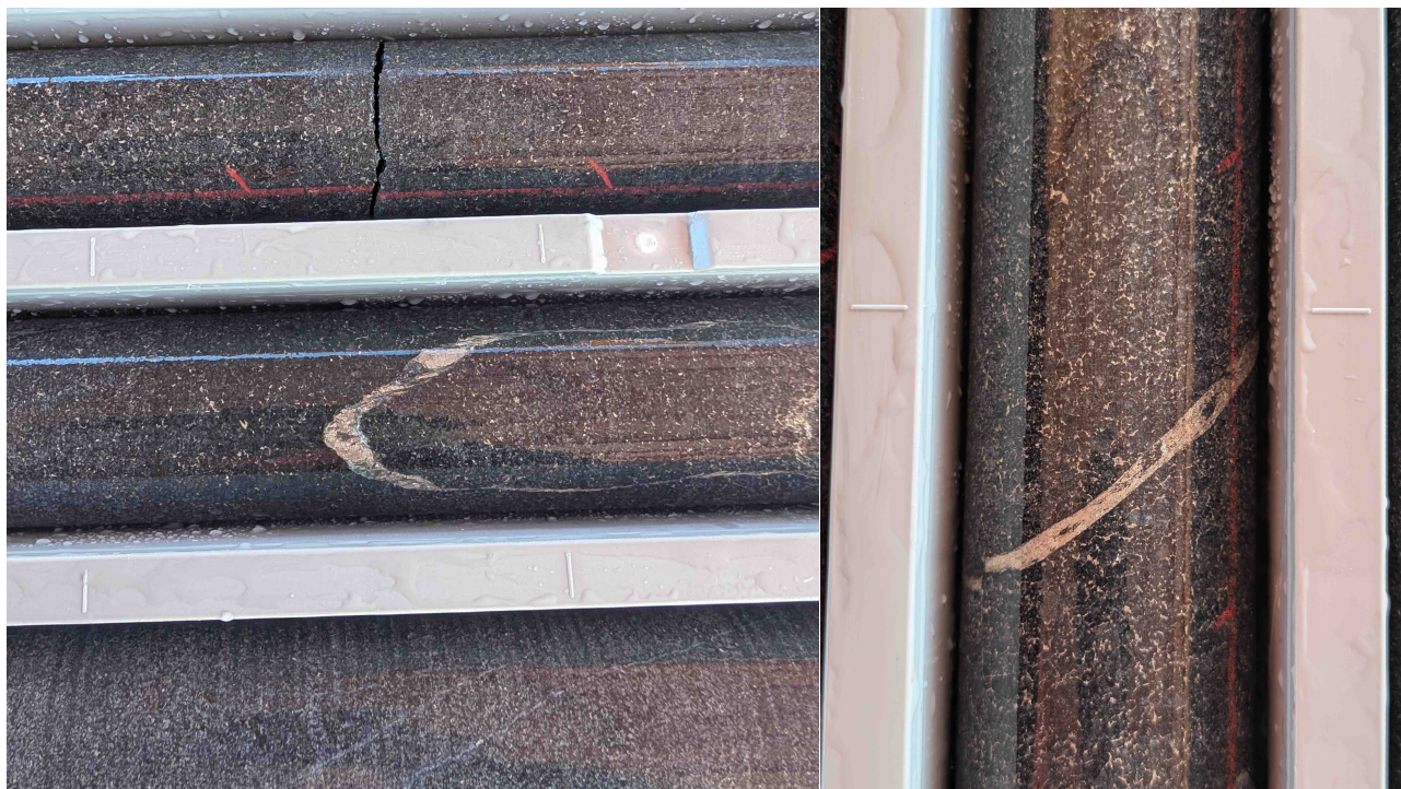
Figure 3: Photos showing examples of heavily disseminated sulphide in hole MTRC009 (EIS9) (left 1355m, right 1350m)
