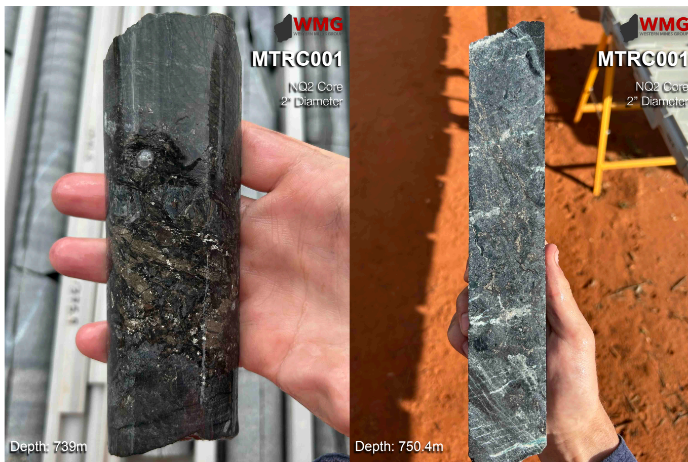
Figure 4: Photos showing examples of sulphide segregations and coarse sulphides in hole MTRC001 Note: core is NQ2 being 2 inches or 50mm diameter
