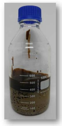
Figure 2 -Xanadu-1 oil and oil-cut mud recovered from 1576.9 mMDRT in the Irwin River Coal Measures "A" sand with the Schlumberger Saturn Probe tool. Oil samples from this zone have been sent for analysis in Perth.
