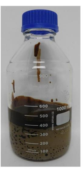
Xanadu-1 oil and oil-cut mud recovered from 1576.9 mMDRT in the Irwin River Coal Measures "A" sand with the Schlumberger Saturn Probe wireline tool. Further oil samples from this zone have been sent for analysis in Perth.
