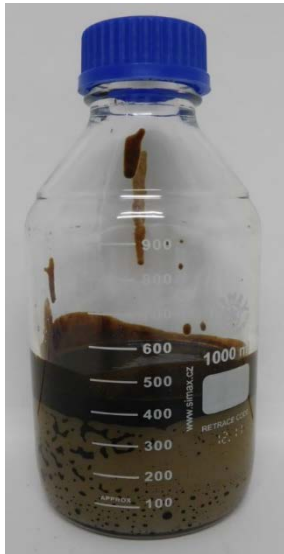
Figure 1 -Xanadu-1 oil and oil-cut mud recovered from 1576.9 mMDRT in the Irwin River Coal Measures "A" sand with the Schlumberger Saturn Probe tool. Oil samples from this zone have been sent for analysis in Perth.
