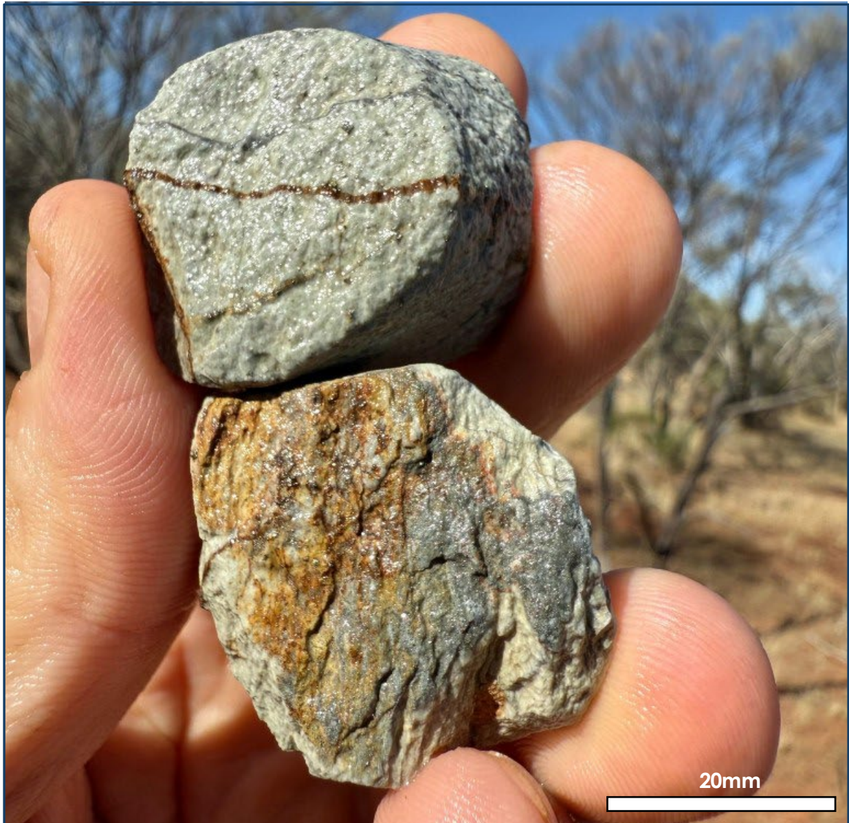
Figure 3: Air-core chips/stubs from 107-108m (bottom-of-hole) of 24IWBAC063 displaying foliated, medium-grained, intermediate (andesitic) volcaniclastic lithology, with strong sericite alteration, up to 3% veining and 5-10% fine disseminated sulphides as a combination of both pyrite and arsenopyrite.
