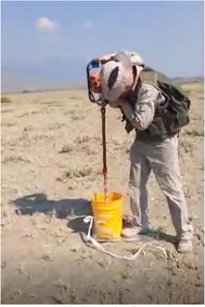
Figure 3: Auger Sampling
