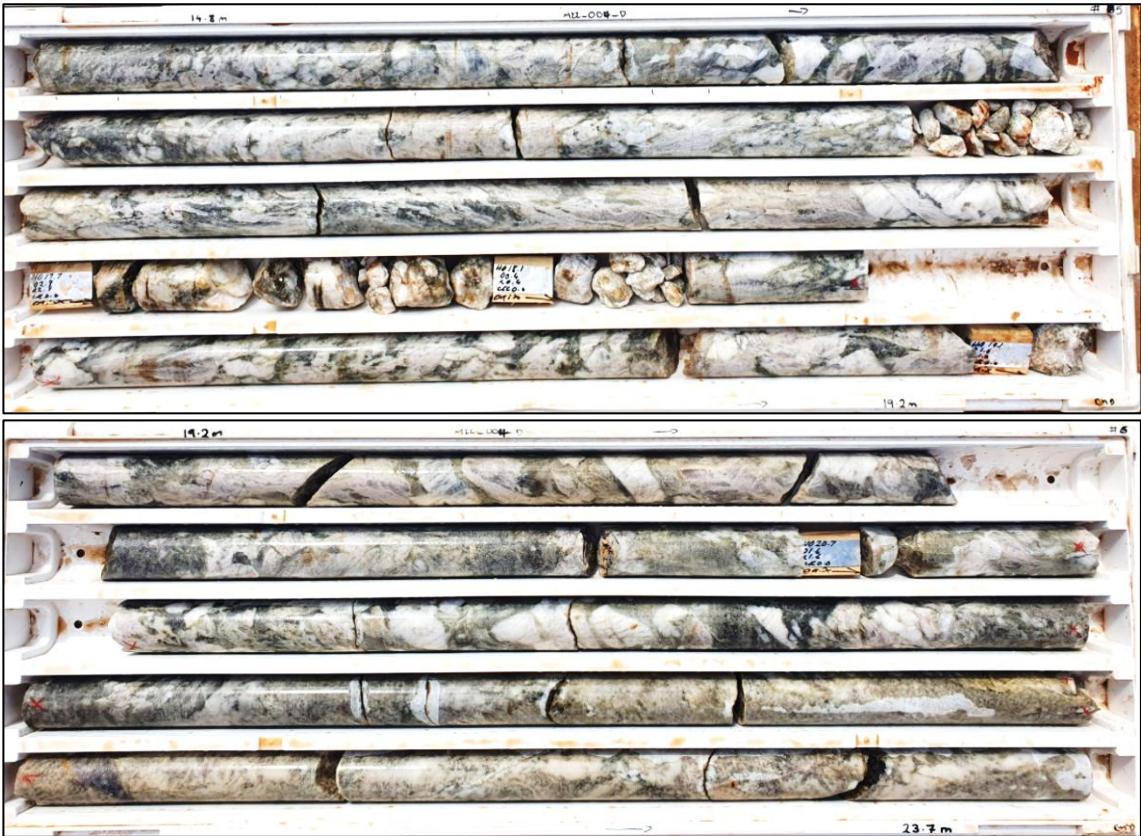
Figure 11: Drillhole M22_004_D: has intersected pegmatite from surface to 57.7m (EOH). The hole was drilled down dip of pegmatite Zone 2. Above are the photos of pegmatite with chlorite, mica and k-feldspar from 14.8m to 27.3m
