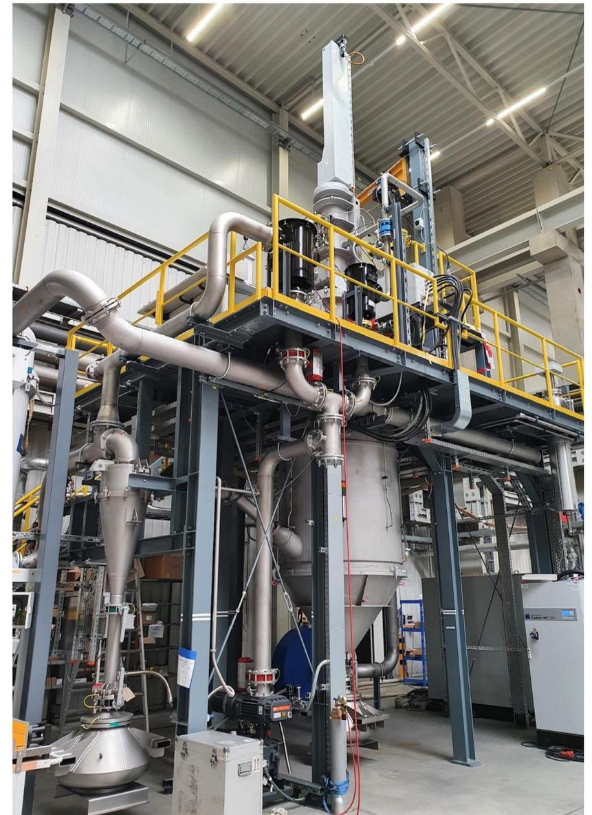
Electrode Inert Gas Atomiser (EIGA)
