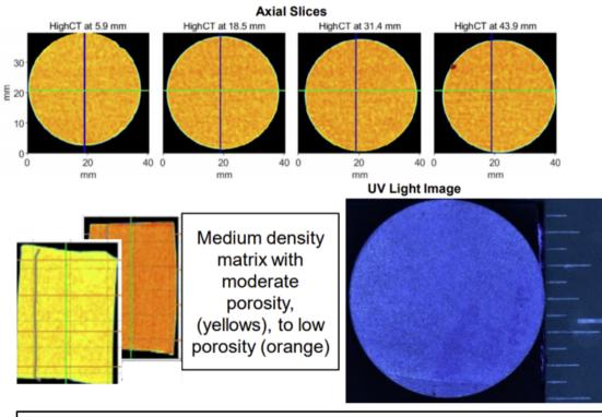
Plug CT scans serve to evaluate the quality of core trims on the basis of their porosity distribution, mineralogy and density. This particular sample exhibits strong fluorescence under UV and is suggestive of moderate porosity. This depth corresponds with one of the two intervals that had oily or 'petroliferous' odours
