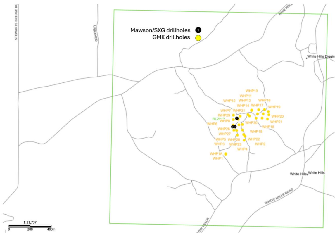
Figure 3 - Historical drilling within EL008807 (source GeoVic) showing 29 reverse circulation drill holes by Gold Mines of Kalgoorlie. An additional three diamond holes were subsequently drilled by Mawson Gold/SXG.
